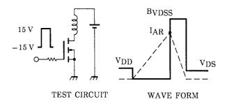
$$\begin{array}{l} T_{ch} = 25^{\circ}\text{C (Initial)} \\ \text{Peak I}_{AR} = 11 \text{ A, R}_{G} = 25 \, \Omega \end{array} \quad E_{AS} = \frac{1}{2} \cdot L \cdot I^{2} \cdot ( \, \frac{B_{VDSS}}{B_{VDSS} - V_{DD}} ) \\ V_{DD} = 24 \, \text{V, L} = 1.0 \, \text{mH} \end{array}$$
